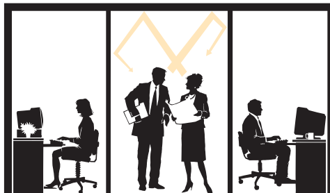
Traditional Closed Office: Sound is repeatedly reflected off all surfaces and absorbed at the ceiling with NRC 0.55 minimum—but these standard ceilings are unacceptable for effective open plan design/call centres
