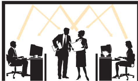
Call Centre Open Plan: Sound is reflected at a single angle over the partial height divider, causing distraction and loss of privacy. Absorbing this angled sound requires a ceiling with a minimum 0.85 NRC.
