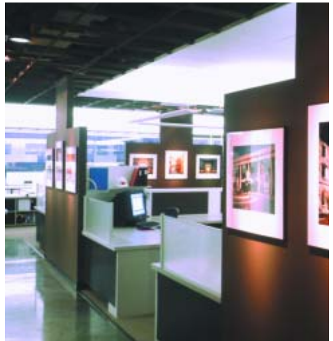
The partially open ceiling design at Newcomb & Boyd's new offices made plenum-based sound masking difficult to implement. It posed no problem for Armstrong's i-ceilings system because the speaker panels are installed in the ceiling plane.
