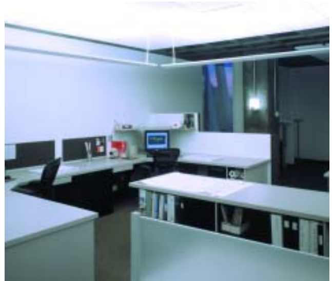
In Newcomb & Boyd's open office plan, acoustical ceiling panels are placed only in those areas located above employee work areas. Each ceiling "cloud" contains an i-ceilings speaker panel to help ensure better speech privacy.
