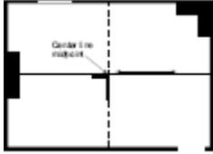
**Step 3.** Leave release paper on back of tile, and position tiles in one quadrant of the room to determine border tile size. Shift the starting line(s) 1/2 the dimension of the tile; i.e.. shift 6" for a 12" tile to maximize border tile size, if necessary.
